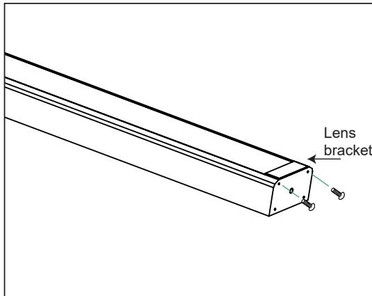
1 Remove two screws from both end caps to remove lens brackets.
