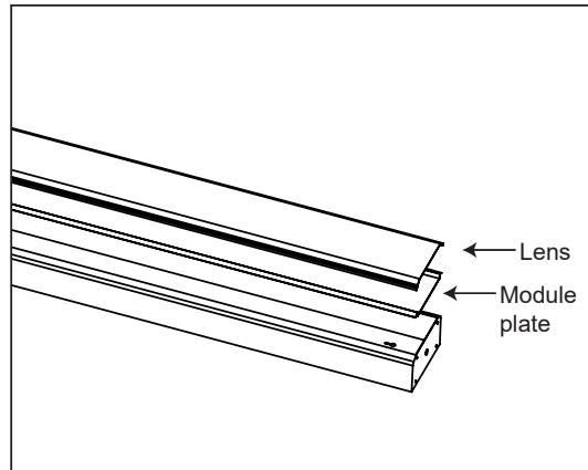
2 Then remove lens and unscrew module plate.
