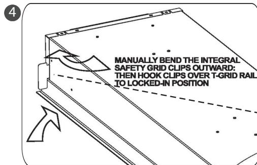
4 Bend the safety grid clips 90° with hand, then secure the clips over T-grid rail to lock-in position. Check to make sure the fixture is firmly fixed on the T-bar grid.
