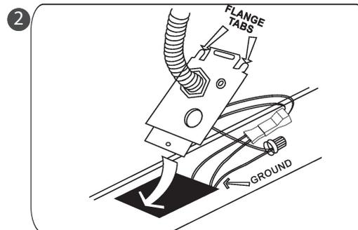
2 Punch a knockout and make proper wiring connections including a ground wire.
