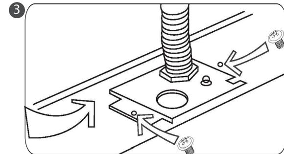
3 Close the access plate and make sure to fix the screws back proper access plate closure.
