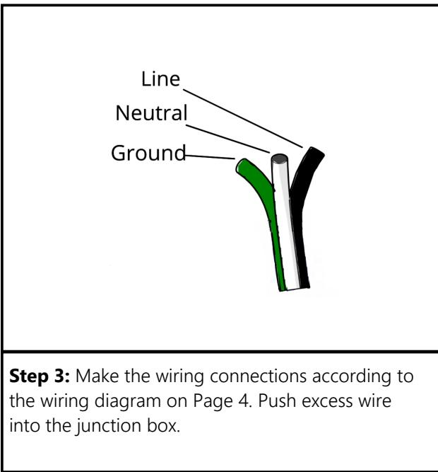
**Step 3:** Make the wiring connections according to the wiring diagram on Page 4. Push excess wire into the junction box.
