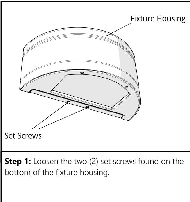
**Step 1:** Loosen the two (2) set screws found on the bottom of the fixture housing.
