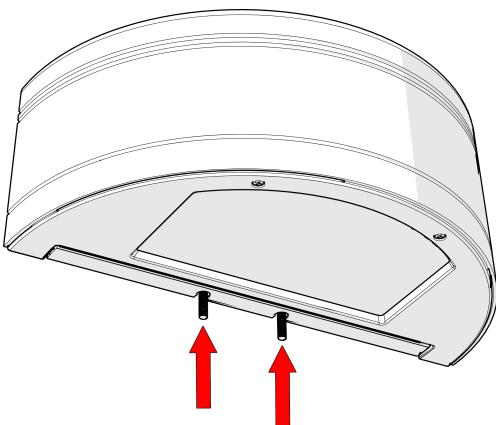
**Step 5:** Tighten the two (2) set screws to secure the fixture housing to the quick mount bracket.
