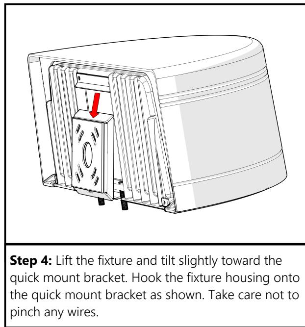
**Step 4:** Lift the fixture and tilt slightly toward the quick mount bracket. Hook the fixture housing onto the quick mount bracket as shown. Take care not to pinch any wires.
