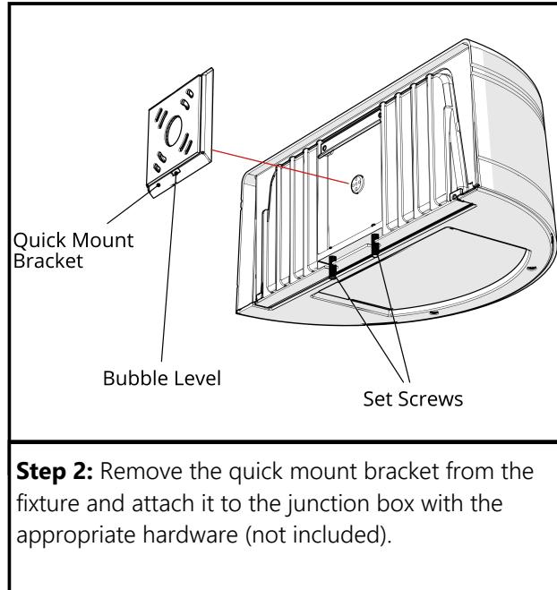
**Step 2:** Remove the quick mount bracket from the fixture and attach it to the junction box with the appropriate hardware (not included).
