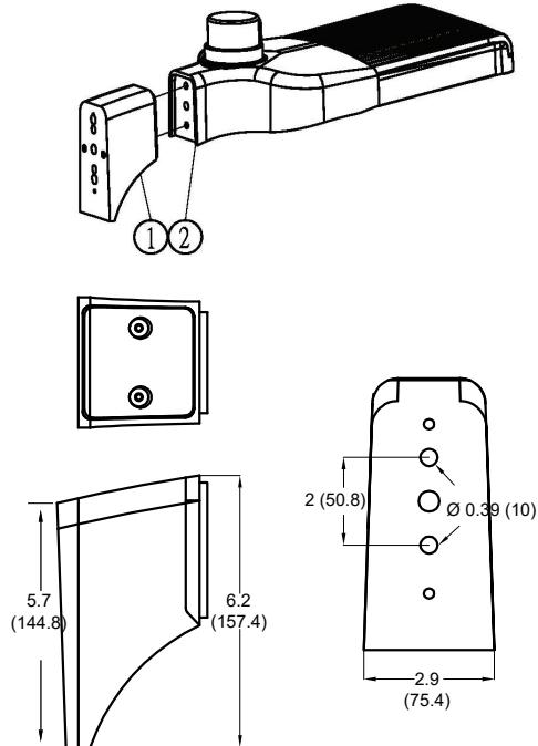
**PMS** : Secure ① and ② together and install the fixture to the square pole.
