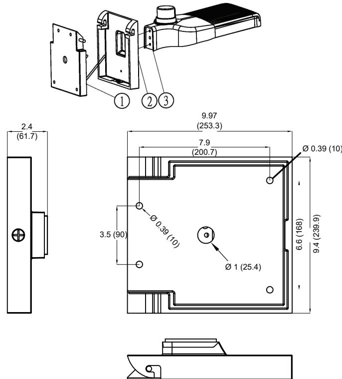
**WM** : Secure ① on the wall with 4 screws, then assemble ② to ③. Finally, install ② + ③ back to ① and secure.
