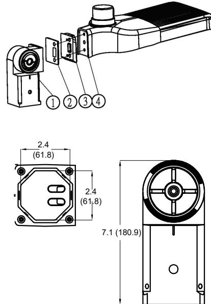
**SF** : Secure ①, ② and ③ together, then attach to ④. Adjustable SF mount available for pipe installation (1-21/32" O.D. to 2-3/8" O.D.).
