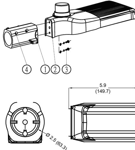
**MA** : Assemble ① and ② together to install onto ③. Fix and secure ④ with 4 screws.
