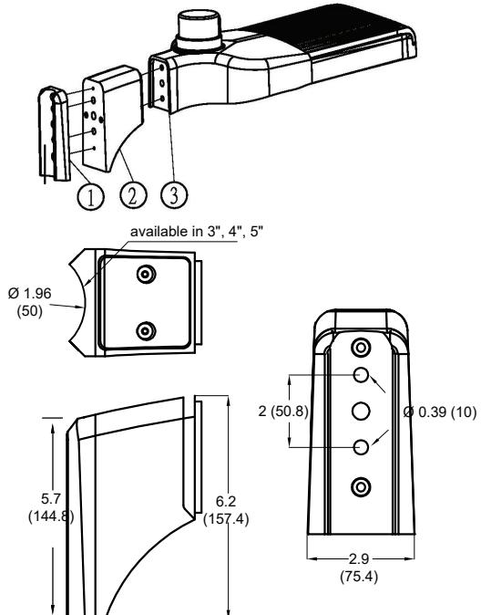
**PMR** : Secure ① and ② together, then attach to ③. Install the fixture to the round pole.
