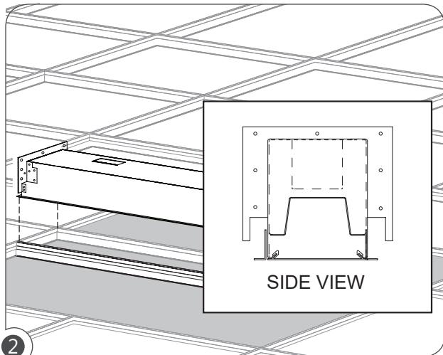
2 Drop fixture on to T-bar ceiling.
