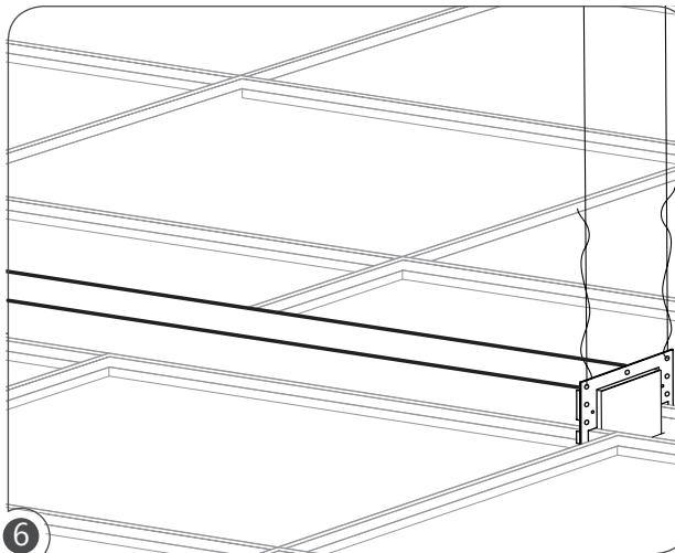
6 Make sure both ends of fixtures is secure with support cable and bracket is properly installed between T-bar grind and fixture.
