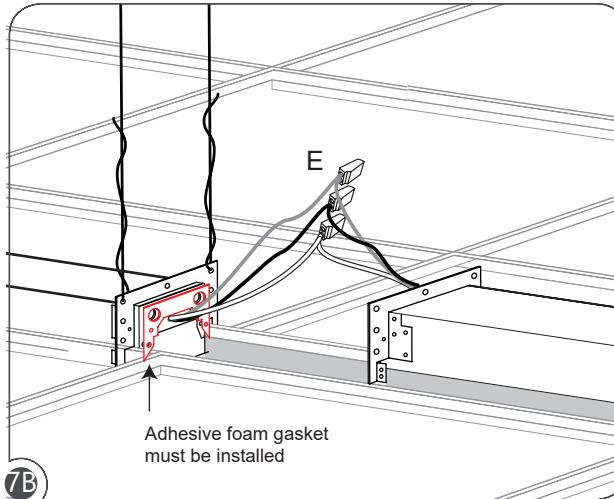
Connect power wire together from each fixture running end to end for continuous row with Wire connectors (E).
