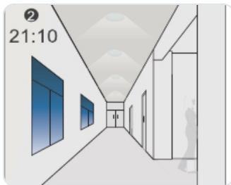
2 · 21:10 The light dims to stand-by level after the hold-time.
