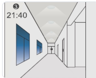
3 · 21:40 The light remains at dimming level at night.
